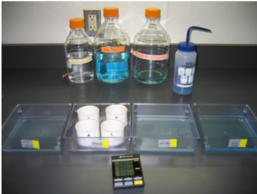
Fig 2. Embryo sanitation station. 5 containers are set-up for 0.5X embryo media, bleach, sodium thiosulfate, pronase, and rinse solutions. Pre-made large volume solutions are shown in the background.
