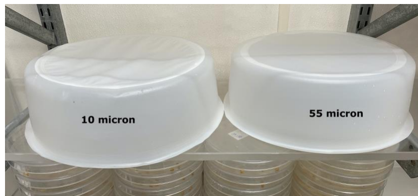
Figure 2. Mesh sieves used in the cleaning and concentrating of paramecia. A 10 µm and 55 µm EZ-Strainer can be obtained from various on-line vendors. To speed the sieving process, a large sieve diameter is recommended. See vendor information below or contact, zirc@zebrafish.org for questions.
